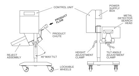
On a standard Pharmaceutical Metal Detector, the control unit is mounted on the stand. A power supply box is secured at the back of the control unit.
