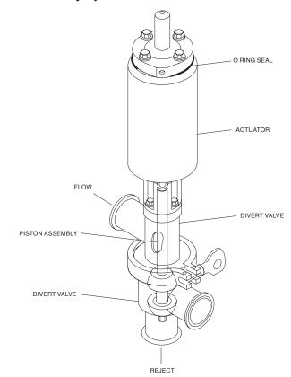
Constructed from 316 stainless steel, the valve comprises a divert valve on which a normally closed spring return pneumatic actuator is mounted. A piston assembly is fitted inside the body. All metallic components are constructed from 316 stainless steel. The recommended air supply pressure is 80psi (5.5 bar).
