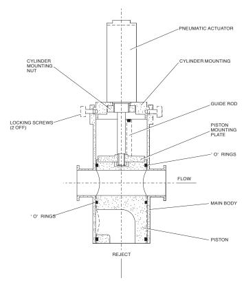
The pneumatically operated, straight-through flow diverter device is constructed from 304L stainless steel. The valve comprises a body with a double acting pneumatic actuator. A piston assembly is fitted inside the body. All metallic components are constructed from either 304L stainless steel or aluminium. The piston is constructed from Acetal co-polymer or polysuliphone.
