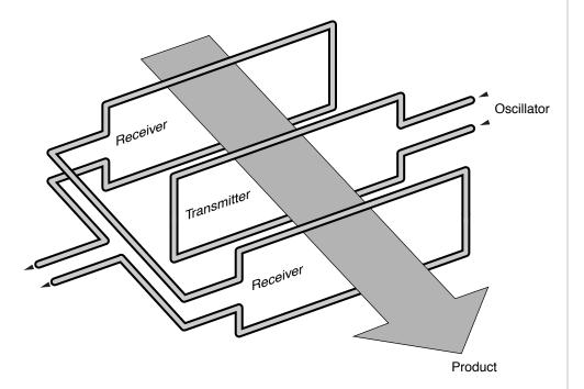
The central coil is referred to as the transmitter coil, and this transmits a radio-frequency signal similar to the frequencies used in AM broadcasting. Spaced equally on each side of the transmitter coil are two receiver coils, which act as aerials to pick up the radio signal. The metal detector measures the difference in voltage between these coils, and this is referred to as the signal.
