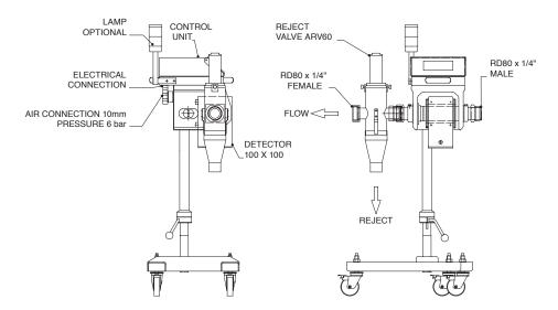
The Pipeline Metal Detector is of stainless steel construction and consists of a pipeline detector assembly and a control unit. An automatic reject valve can optionally be fitted. The pipeline detector assembly consists of a pipeline body, which contains a removable Acetal product pipe, and a search head.
