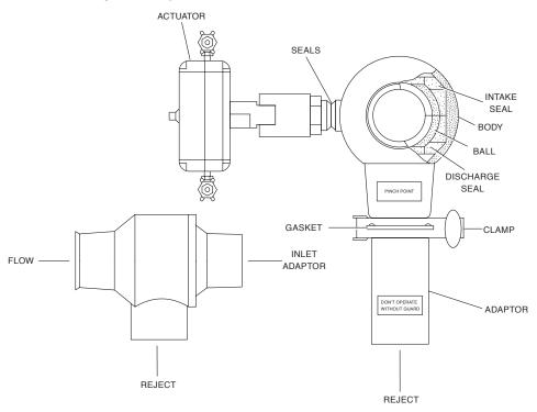
The unit comprises a valve body with integral 'T' ball connected to a modified actuator. All metallic components are constructed from 316 stainless steel, with teflon (or Mica filled) seals and Buna-N O rings. The recommended air supply pressure is 100psi (6.9 bar).
