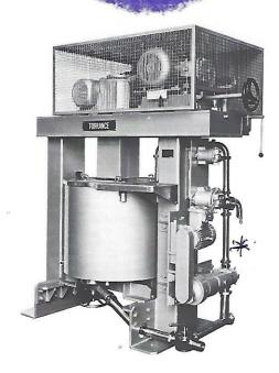
The 100SM Attritor has a jacketed stainless steel grinding vessel. The built-in pumping and circulating system, with quick release couplings for easy cleaning, facilitates recirculation during processing in order to shorten dispersing time and increase the volume of process material. It can also be used for charging and discharging the vessel.
